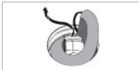
Fig. 8.6 Removing the activated charcoal filter through the inlet opening
